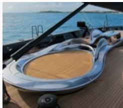
Deck structure and carbon fibre steering pedestals on the 130' Wally sailboat
